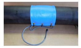
Install Treatment Pads Opposing Each Other with labels "To Pipe" facing the pipe.
